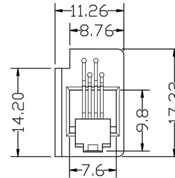
Tolerance for jack:  $\pm 0.2\text{mm}$
